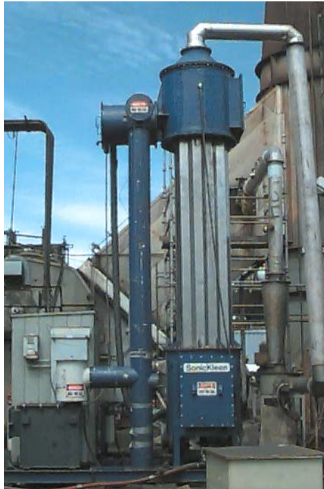
Figure 10. Pilot WESP used for testing at Elk Falls.
